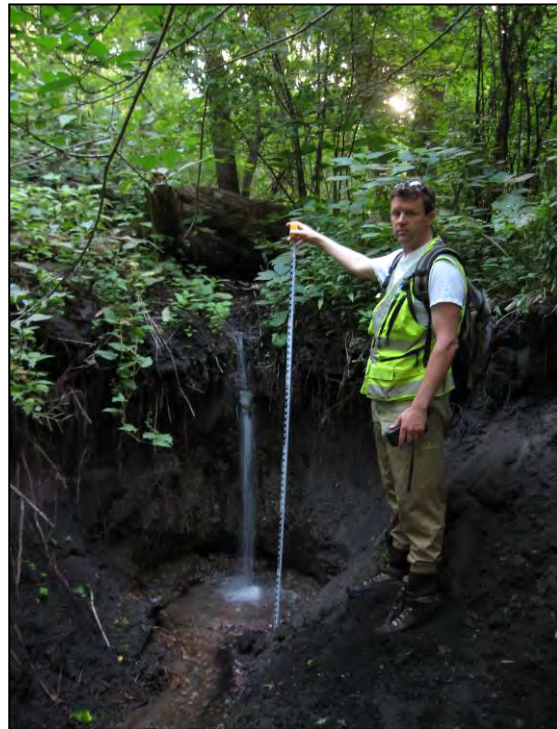
Figure A-2: A headcut and incised channel on a small stream in Scott County.
