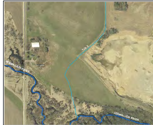
Figure C-13, Tributary 3: Air photo of the Tributary 3 alignment with no visible channel bed or banks. A shallow swale through the fields carries overland runoff to the Vermillion River, but no channel features are apparent.
