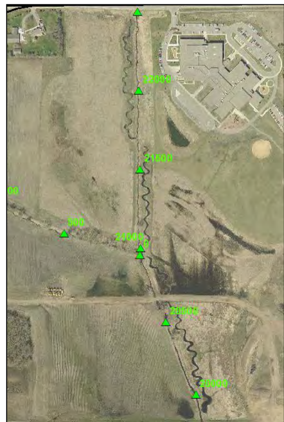
Figure 10: Middle Creek showing the sinuous restored channel that has not been activated. Water still flows through the straightened ditch. The large building in the upper right is the Farmington Elementary School.
