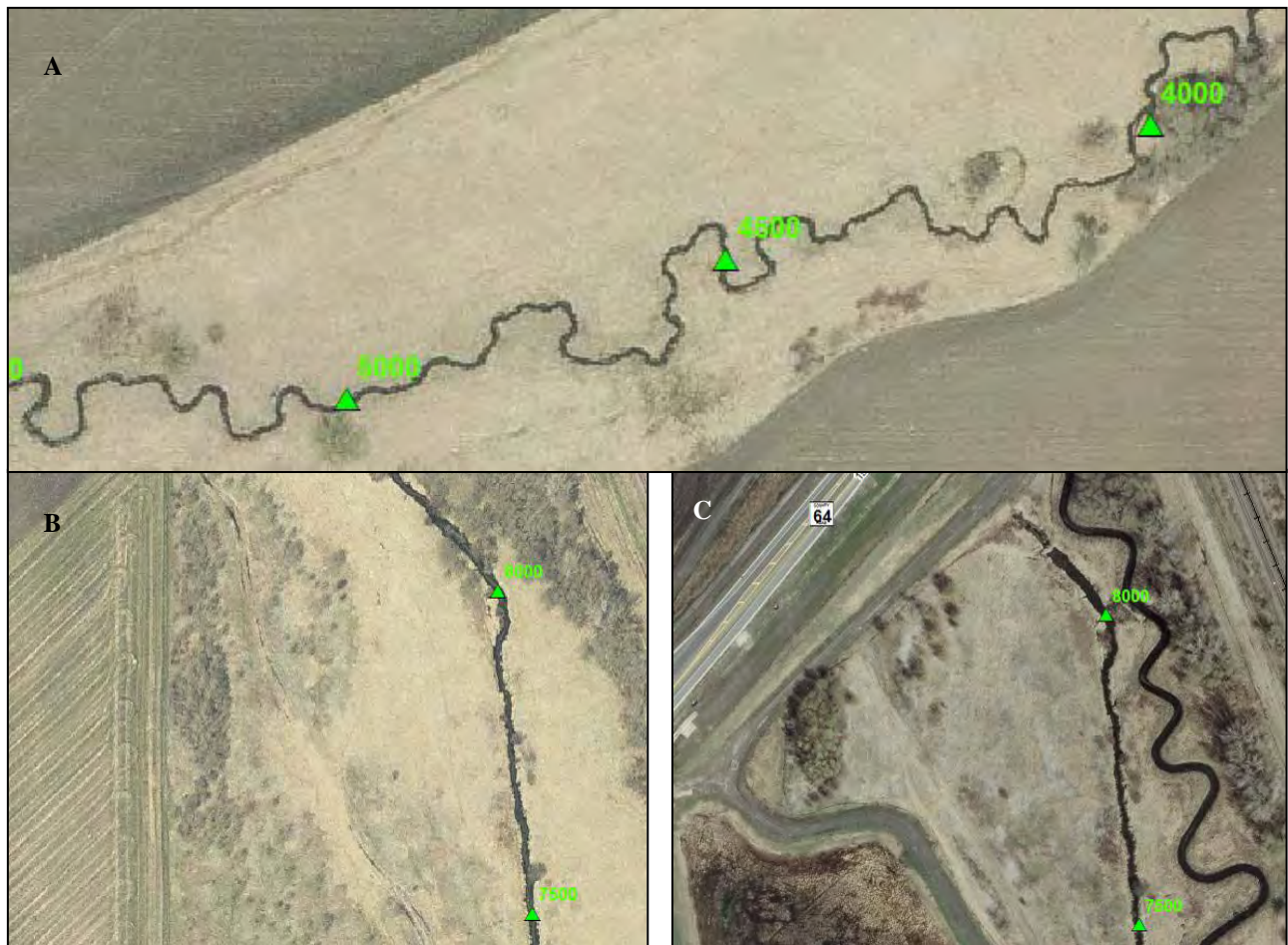
Figure 13: (A) Lower Middle Creek showing sinuous channel left largely untouched since settlement demand in the mid-1800s. North Creek (B) before and (C) after restoration. The sinuosity and channel geometry is more uniform that on Middle Creek, but the meander width and wavelength are similar.
