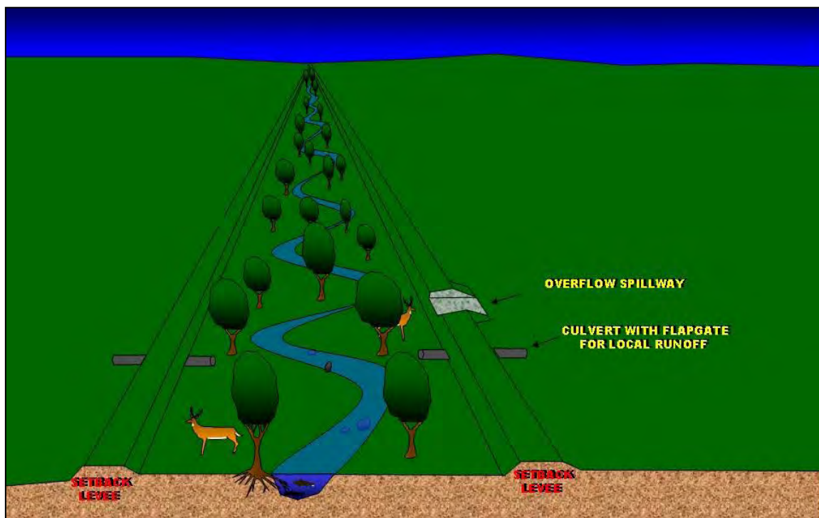
Figure B-9: Restoration of a ditch within levees to create a meandering stream with a vegetated riparian buffer (courtesy of L. Aadland, MN DNR).
