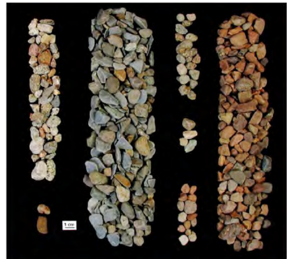
Figure 7. The Cromwell Formation includes rock types of the Superior Provenance that are more durable and less reactive than those of the New Ulm Formation and are favored by the aggregate industry. https://www.mn.gov/pebbles.htm
