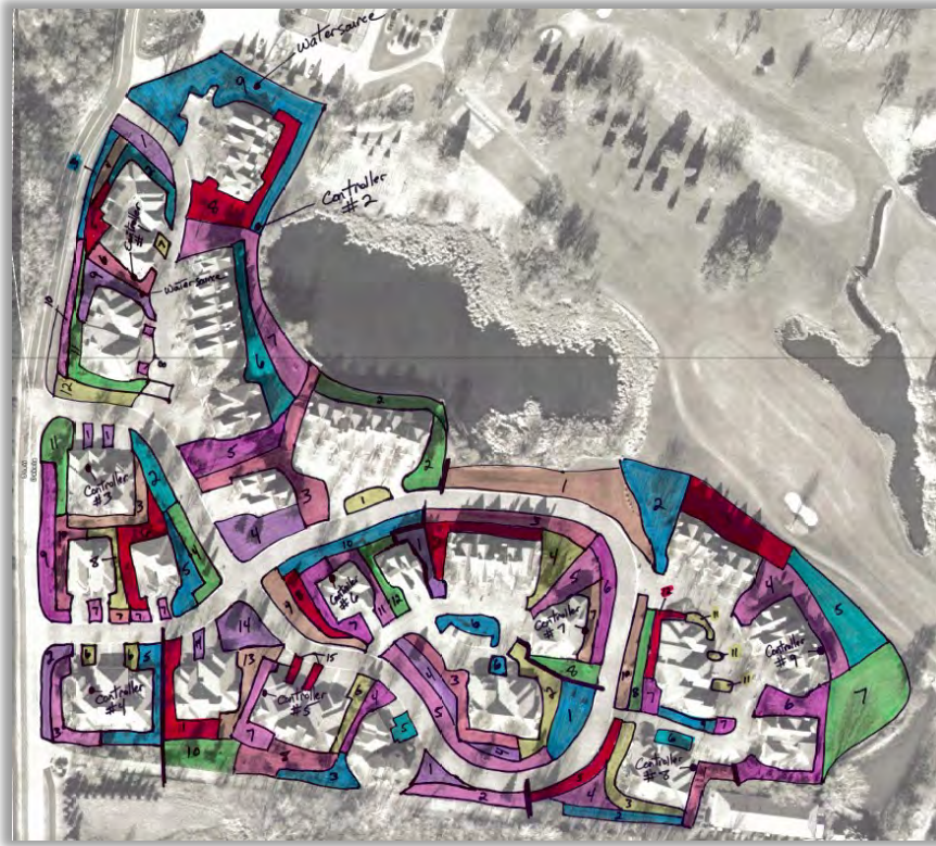
Figure 1. Mapped irrigation zones. Controllers installed on residential homes have the capabilities to connect to in-home Wi-Fi.
