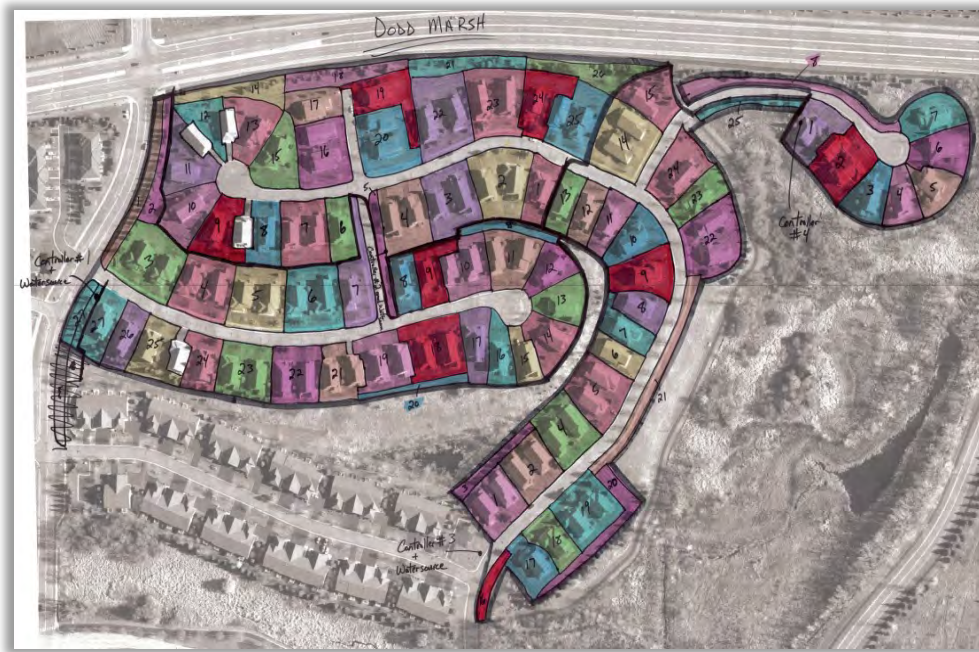
Figure 1. Mapped irrigation zones. Zones are seen to irrigate greenspace according to single family home property boundaries (with some zones irrigating two home properties).
