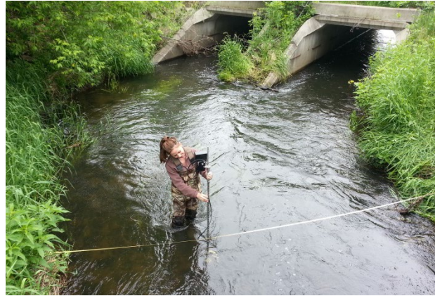
DCSWCD staff measuring flow at the NC808 monitoring site
