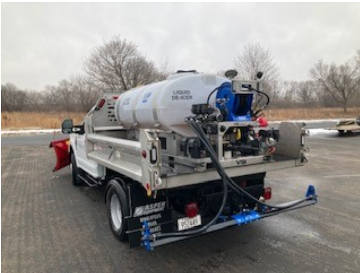
Figure 2. Back side of a City of Rosemount truck with new de-icing equipment installed.
