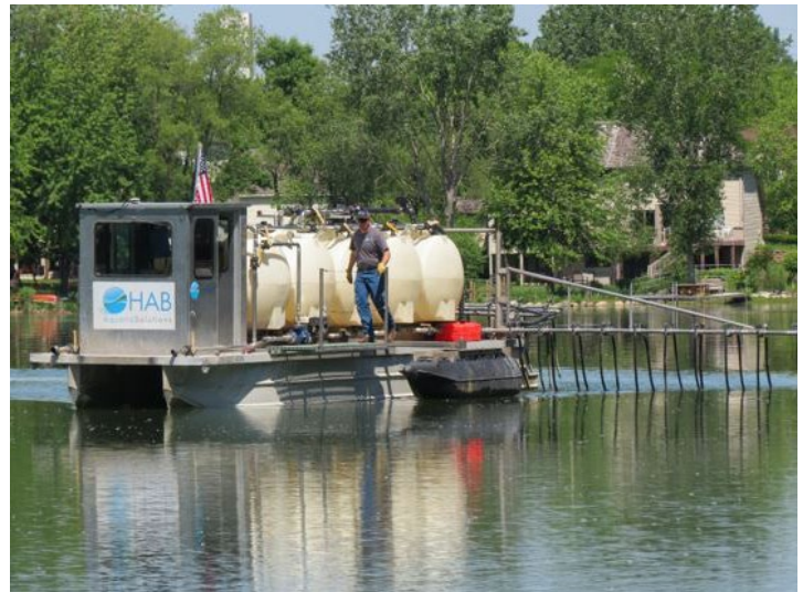
Figure 3. Application of alum in a lake using a barge
