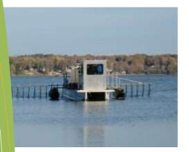
A boat with equipment, similar to this, applied alum to regional stormwater ponds in Burnsville to reduce the amount of phosphorus available for algae growth.
