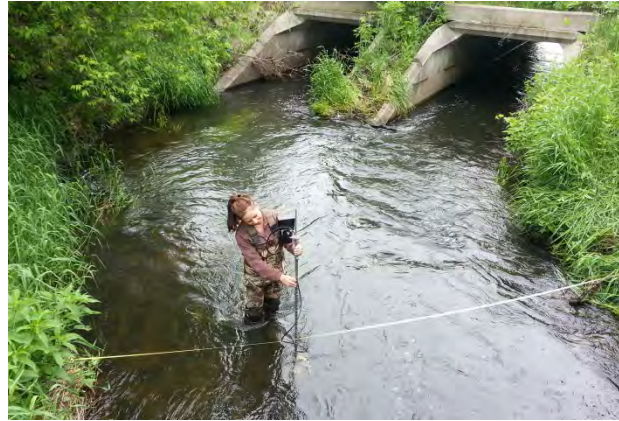
DCSWCD staff measuring flow at the NC808 monitoring site Photo Credit – J. Van Der Werff Wilson
