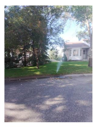
Sta 10 – sprinklers in front & side of 15969 Suggest nozzle balance the entire station. Change the large area rotor sprinklers in the front yard to smaller style sprinklers. Add a sprinkler at the drive corner.
