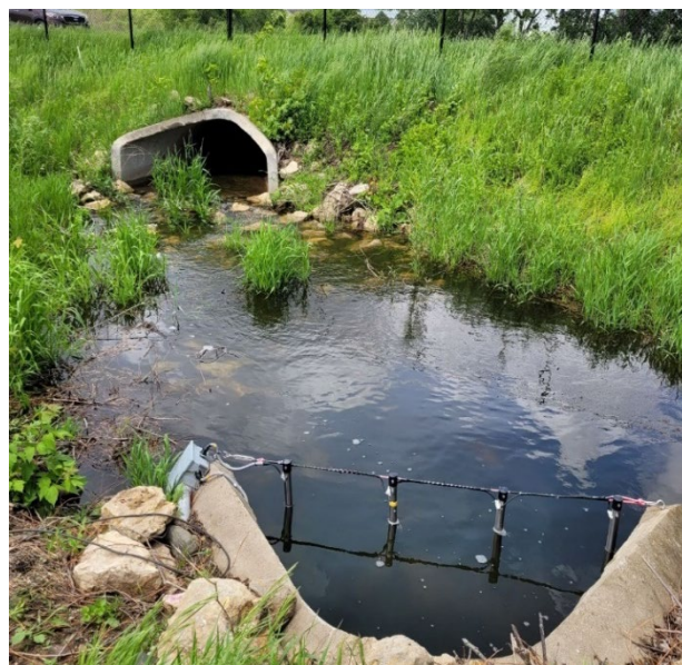
The low-voltage electric barrier deterring invasive fish from moving between East Lake and North Creek.
